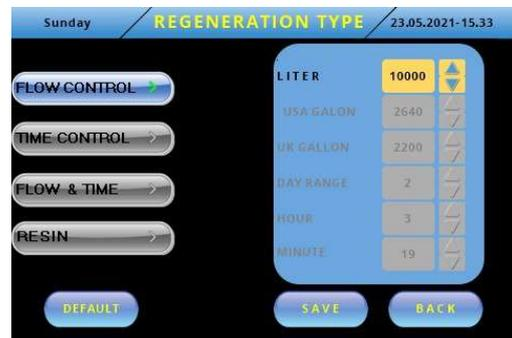
After selecting Volume Control (which is total volume treated before regeneration occurs), press the save button. Liters, US Gallons, Imperial Gallons will be displayed to select the unit of Volume. Select one of them and press the save button. If you do not make a selection, the Liter application will be saved, Liter is the factory setting (default).
