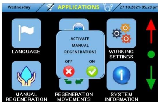
This mode regenerates the treatment device manually. When you press the manual button, the values you have made in the operating settings and operating information are displayed on the screen. When you press the accept button, the device starts regeneration manually. If you want to make changes, make the change you want by pressing the back button, then start the Manual Regeneration process by pressing the accept button. The colored round image starts to rotate.
