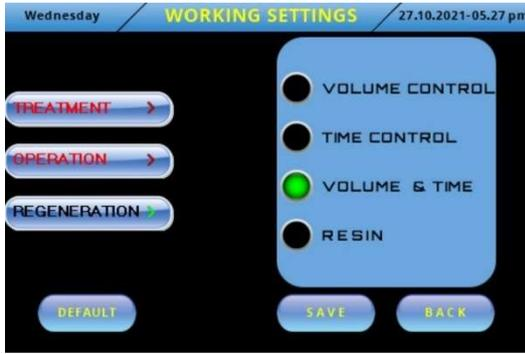
Select “Regeneration” from the Working Settings screen. You can regenerate the treatment device according to volume control, time control, volume & time control and resin amount. If you do not make a selection, the factory default Volume Control application is saved.
