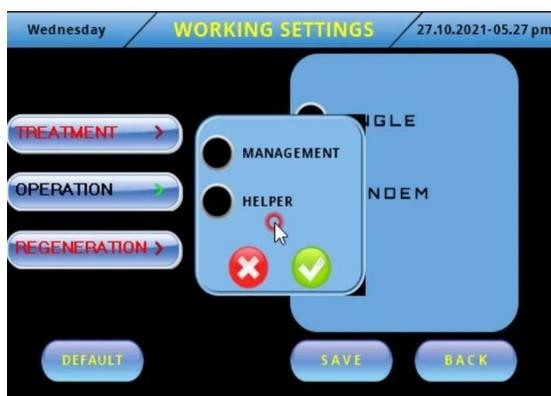
When the "Management" valve switches from the service section to regeneration, it sends a command to the "Helper" valve, allowing it to go into service.
