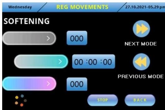
It functions to control and inform regeneration cycles during Service or Regeneration. When you press the regeneration cycles button, the treatment type of the device is written at the top. When the regeneration process starts, the colored round image
