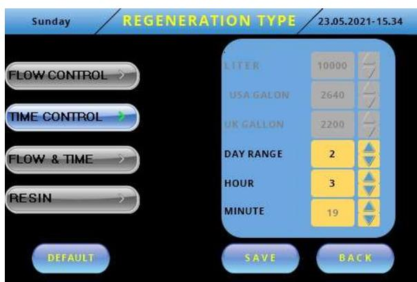
For the Time Control setting, the day range, hour and minute sections will be displayed on the screen. By default;
