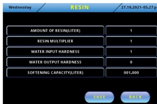
The regeneration of the treatment device will be determined by the resin capacity. Make your selection by pressing the Resin button and press the save button.
