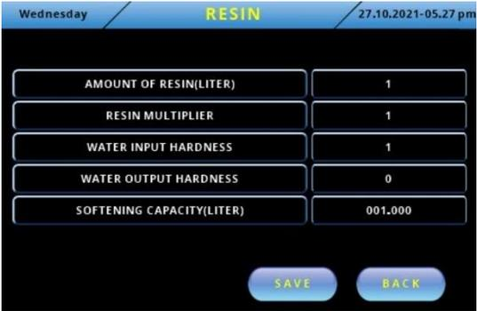
The regeneration of the treatment device will be determined by the resin capacity. Make your selection by pressing the Resin button and press the save button.
