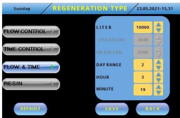
Make your selection by pressing the Volume & Time button. Press the Save button, the treatment device both treats the amount of the adjusted volume and executes the regeneration with the arrival of the set time (day, hour, minute). In other words, whichever of these two conditions fulfill first, regeneration starts accordingly.
