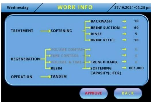
After all the settings are made and saved, the information of all settings you have made in operation type are displayed on the screen.
