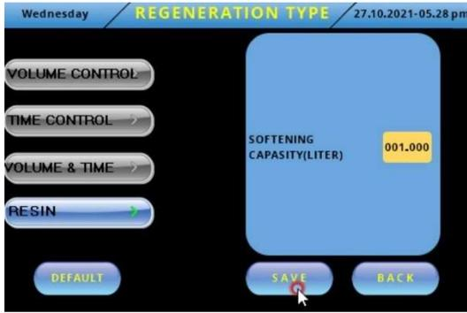
The factory setting (default) is saved as French hardness. When you make your selection and press the save button, the above screen will appear. The respective values are the maximum and minimum ranges;
